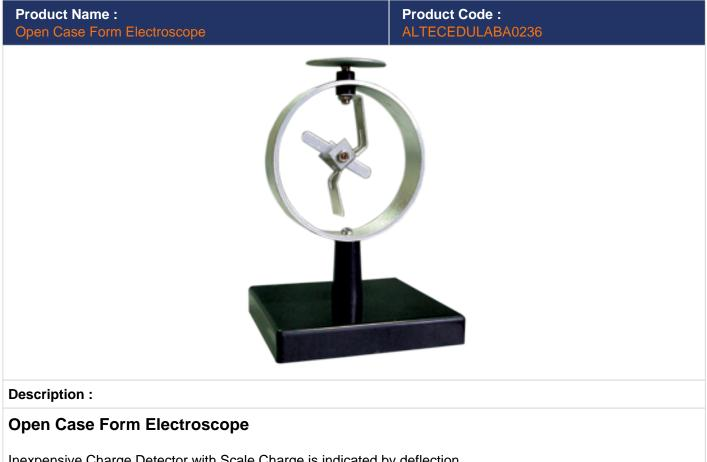
Inexpensive Charge Detector with Scale Charge is indicated by deflection of an aluminized plastic straw which rotates freely on the saddle of the conducting rod. The conducting rod is recessed in the metal housing to shield against air currents.
