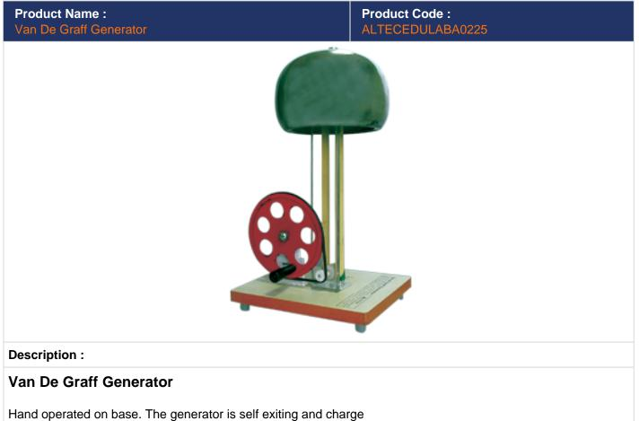
separation occurs. A metal sphere surrounds the upper pulley assembly and charge accumulates on the sphere, which is insulated by a plastic column supporting the pulley assembly. The charge builds up untill electrical breakdown of air surrounding the sphere occurs. Supplied with a discharging sphere
