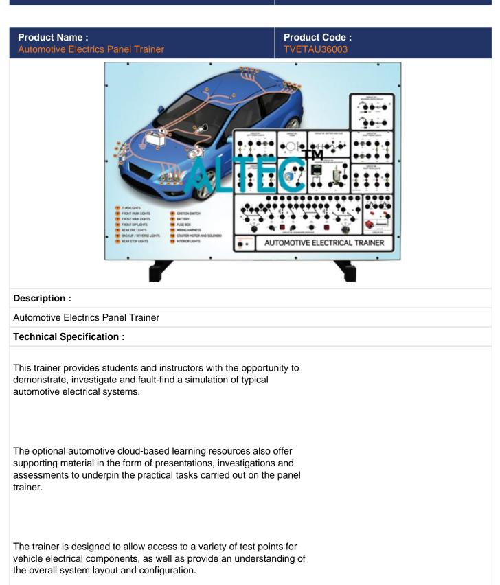
To facilitate the development of techniques in diagnostics and fault-finding skills, the panel includes a range of fault-insertion options to simulate typical real-world system malfunctions.
