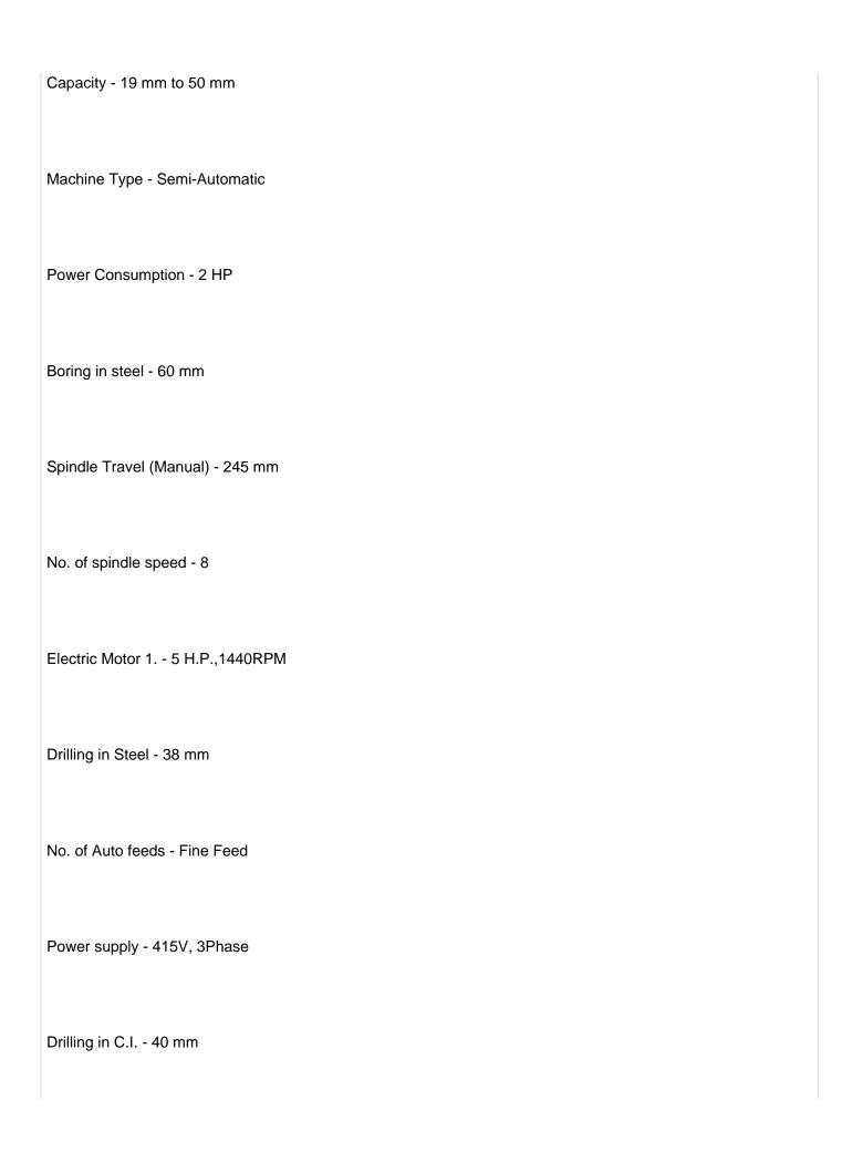
Tapping capacity in steel - 25 mm
